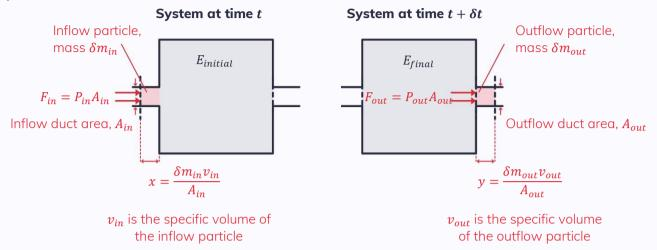
Everything that is shaded grey is the closed system, and the red part is a minute particle entering/exiting the closed system.
